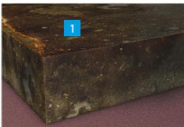
substrate must be sound and absorptive and should furthermore be free of Alkaline Silica Reactive or sulphurous compounds. Any type of surface contamination such as adhesives, adhesive residue, old coatings, curing compounds and underlayments must be removed completely by shot blasting prior to the ORS treatment being applied.
