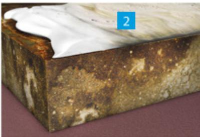
operations begin. This phase uses hot water and a deck spinner washer to clean the surface from the oil that has been washed out and the remaining foam. After the rinse a squeegee and a vacuum is used to remove all standing water from the area to be coated. Depending on the level of contamination more KÖSTER ORS-D treatments can be necessary.
