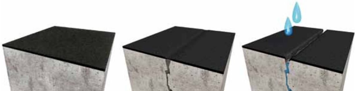
1. Elastic but not crack bridging: The waterproofing layer does not withstand the permanent water pressure.
