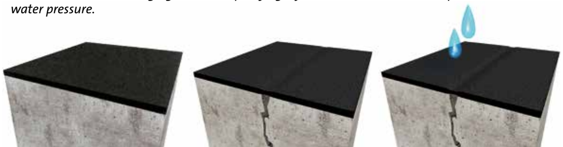
2. Crack bridging waterproofing: In this case due to elasticity and layer thickness. The waterproofing layer withstands permanent water pressure.
