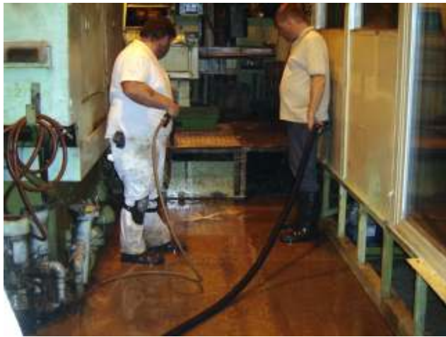
Performing rinse operations to remove all the excess water and oil emulsion prior to the second application of foam.
