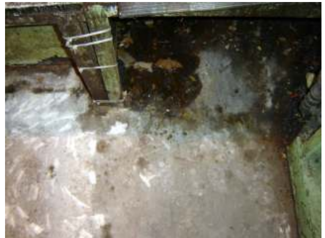
Another area under the machine showing extensive oil build-up under and around these machines.
