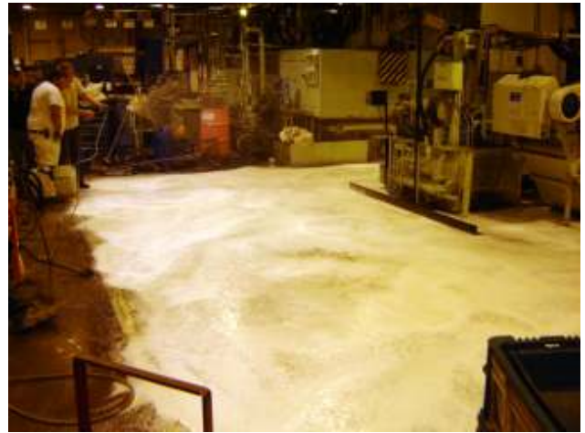
First application of the ORS-D foam complete. At this point the entire area is covered with the carpet and is of a white color. Let this soak in for 1 hour.
