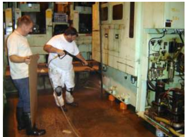
Final rinsing continues. Some spot cleaning with the ORS-D may be necessary and it is a good idea to have some in a small spray bottle to accomplish this application.
