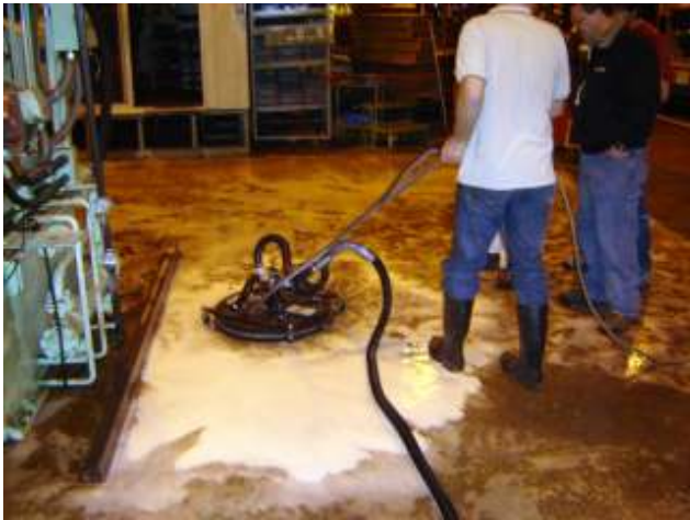
High pressure floor spinner in operation. Pressure is 5000 psi and water is 200° F. Note vacuum hose attachment to help the waste water.
