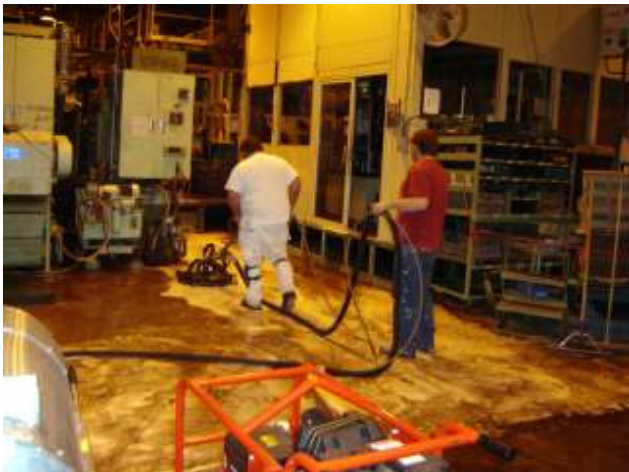
Spinning operations continuing. Note Tom tending the hoses for Junior as he moves the spinner over the entire floor being careful not to miss any spots.
