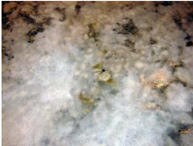
Oil is captured by the detergent and brought to the surface as seen by the yellowish colored areas in the foam above.
