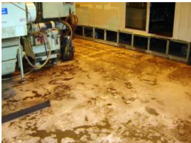
Overall view of the foam as the hour draws to a close. Again notice how the foam is turning clear from its original white color.
