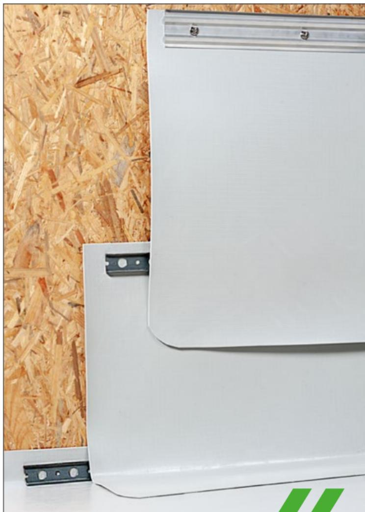
Alternatively, the membrane can also be adhered to the entire surface with KÖSTER Contact Adhesive. The contact adhesive must be applied over the entire surface both to the component and to the membrane to be bonded. The adhesive must dry briefly, this can be checked with a finger test. The glue must no longer pull threads.
